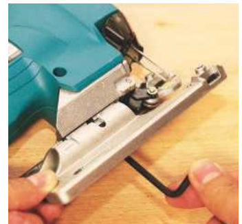
▲ Base tilts are set with the supplied on-board hex wrench
